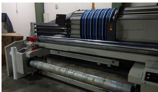
CCI's LUTAN v5.0 and v3.6, Single-end Warping Machine, installed in Huaw Lon's factory
