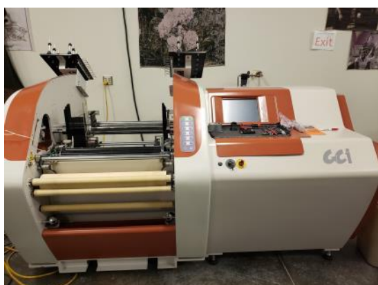
CCI’s SL8900 & The Studio (Sampling Loom), installed in NC State University’s Wilson College of Textiles
