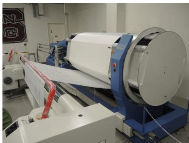
CCI's LUTAN v3.6 (Single-end Warping Machine), installed in NC State University's Wilson College of Textiles
