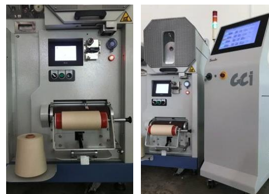
CCI Taroko Multi-spindle Sizing Machine
